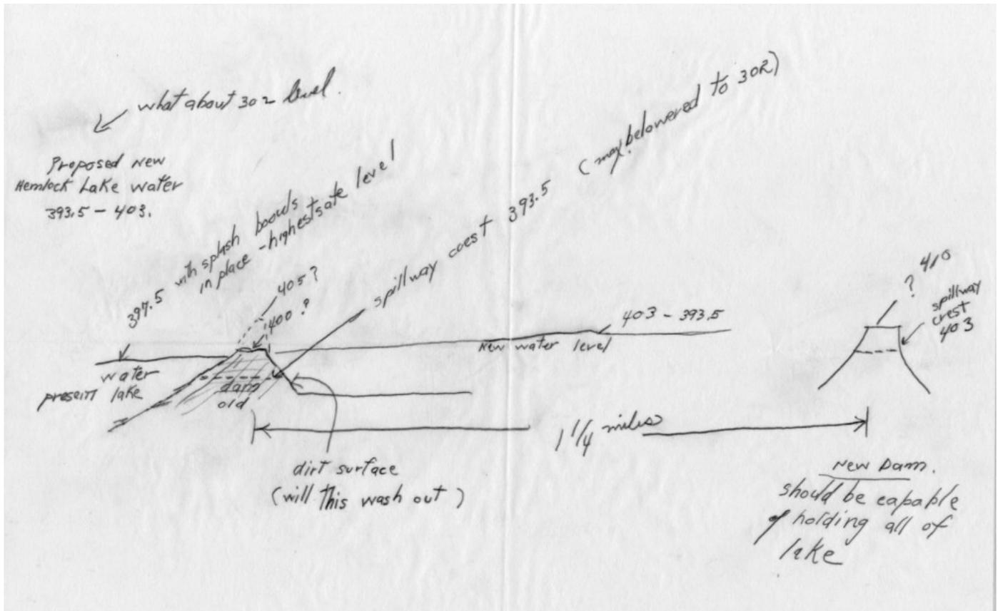
The spillway weir crest at the present Hemlock Lake dam is at elevation 393.5. The drop timbers in the spillway would be removed and the present Hemlock Lake dam retained, but with water at elevation between 393.5 and 403.00, water would stand at the same elevation above and below the dam, and the present spillway would no longer be used as a spillway but merely as an outlet channel.
